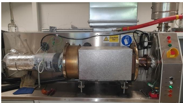
Figure 3. Test section of the DPG test system and the single DPF cassette reactor.
