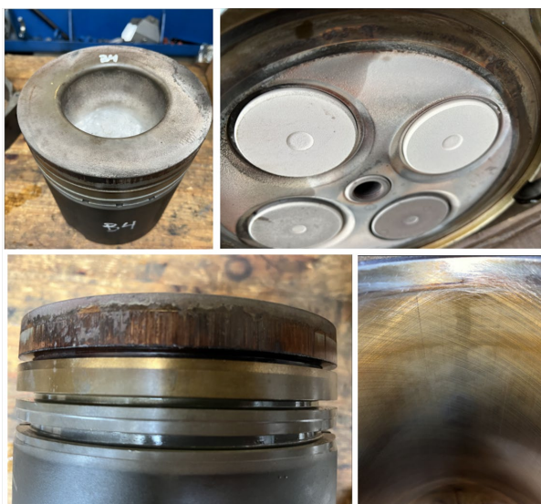
Figure 6.20. Inspection of Cylinder Head, Piston and liner show less deposits and it confirms the high performance of the used Mysella S7 N Ultra 40 in the Gas Engine MWM Caterpillar TCG 2020 V12 (BMEP 21.5bar)
