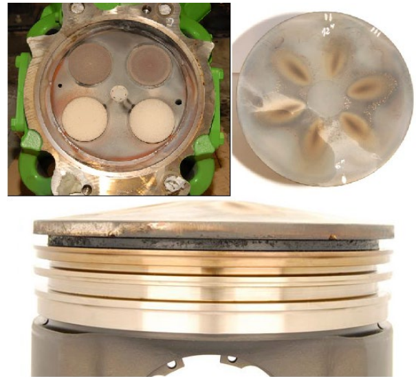
Figure 6.13. Inspection of Cylinder Head and Piston show less deposits, and it confirms the high performance of the used Mysella S7 N Ultra 40 in the Gas Engine INNIO Jenbacher J624 – 24bar (Steel Piston).
