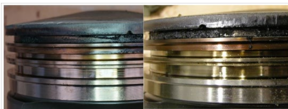
Figure 4. Impressions of piston deposits in J6F engines for a commercial oil blended in API group I base oil (left) and a commercial product blended in group II base oil (right) after similar engine running hours. Oil change has been changed at least twice as frequently with the API group I base oil lubricant.
