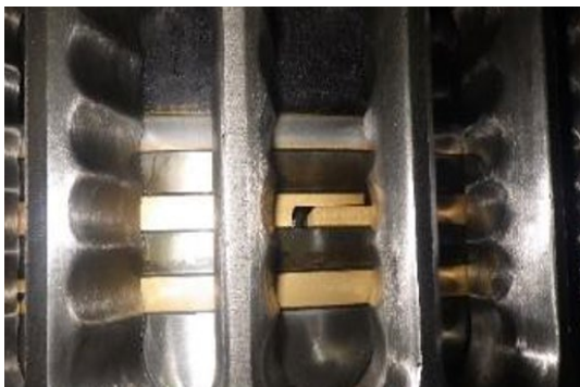
Figure 9. Piston ring packs after 2,000 hours with zero deposits, only slight discoloration on piston ring lands
