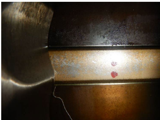
Figure 20. Close up of first piston ring lands in a ME-GI engine operating on Shell Alexia 40 XC with slight deposits on the piston ring lands.
