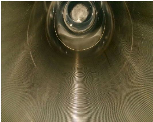
Figure 10. Clear wave cut marks on cylinder liner.
