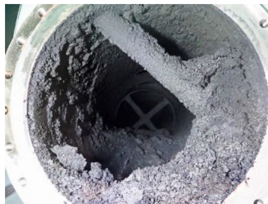
Figure 5. Accumulation of calcium deposits along the exhaust gas path
