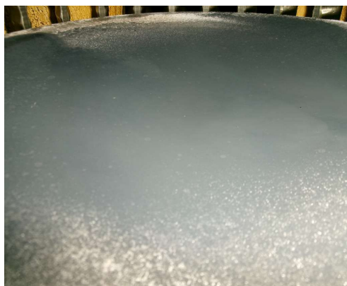
Figure 11. Only minor calcium carbonate deposits found on piston crown.
