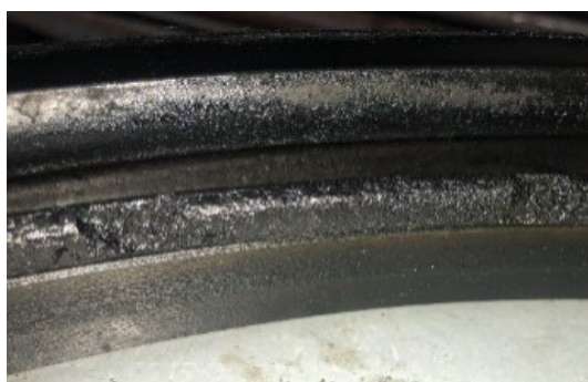
Figure 3. Heavy carbon deposits on the back side of piston rings can lead to collapsed piston rings and scuffing.
