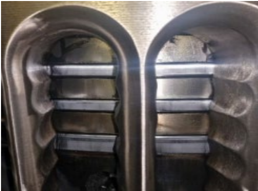
Figure 16. Piston ring lands showing zero deposits after approximately 3,500 hours using Shell Alexia 40 XC with 0.8 g/kWh feed rate.
