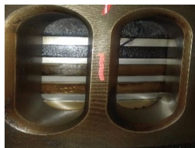
Figure 12. Piston ring lands with deposits (rough surface) and discolorations, running on 100% VLSFO with Shell Alexia 40.
