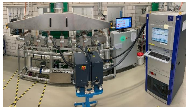
Figure 1. Test bench for catalytic benchmark experiments
