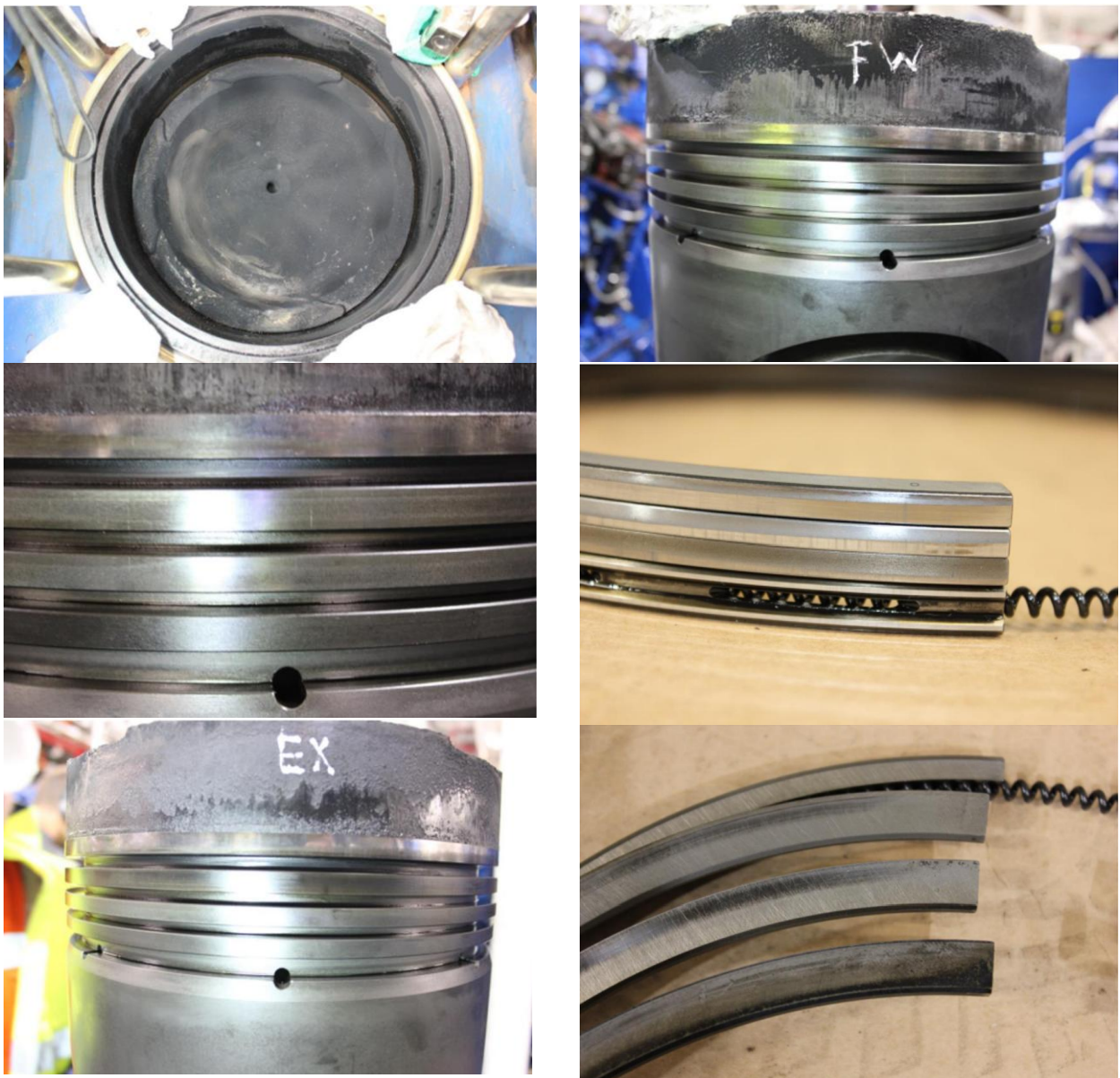
Figure 9: inspection after operation on low SAPS oil.
