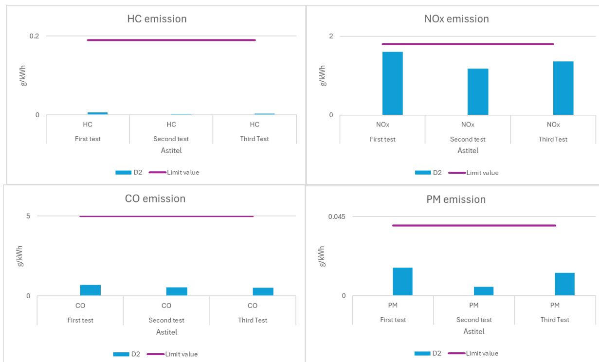
Figure 13: HC, NO x , CO and PM emissions measured during start, mid and end of test.
