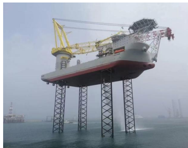
Figure 2: JDN jack-up installation vessel
