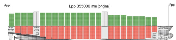
Figure 19. Potential lay-out of cargo spaces to determine container carrying capacity: 15000 TEU.
