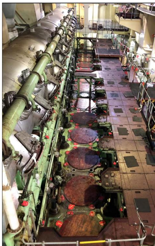
Figure 5. Engine's status after dismantling the RT-Flex96C-B components.
