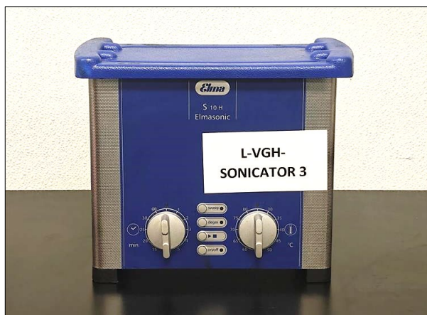
Figure 1 shows a typical lab heated sonicator with dial adjustments for temperature and time.
