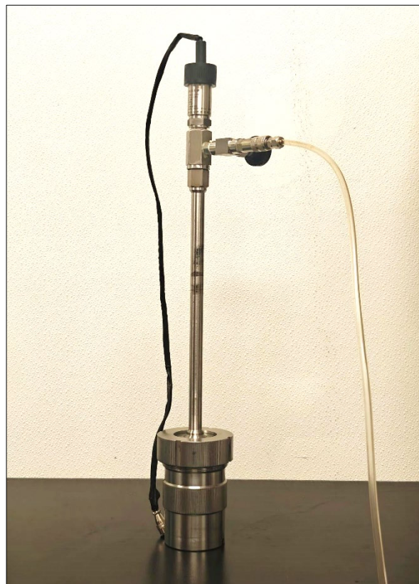
Figure 2 shows a typical oxidation vessel bomb used in ASTM D2272.
