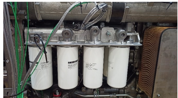
Figure 4 Oil filters connected to the engine
