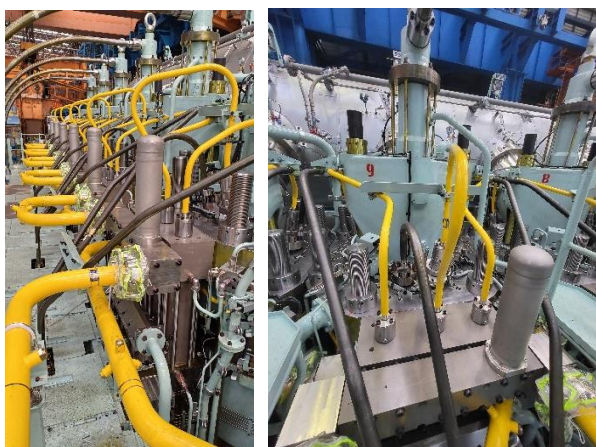
Figure 10. Application of the methanol injection system on the first WinGD X-DF-M (10X92DF-M-1.0) engine.
