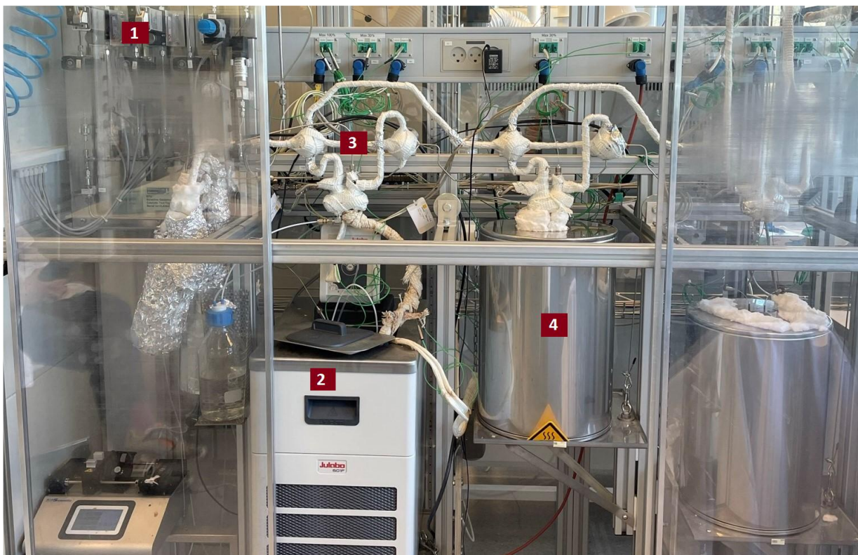
Figure 1. Reactor setup for testing the powder catalysts. The numbered sections in the figure refer to: 1) mass flow controllers for the feed gases, 2) bubbling set up (evaporator) for introducing \text{H}_2\text{O} in the feed, 3) heat-traced and insulated tubes for gas flow, and 4) furnace with the reactor contained within.
