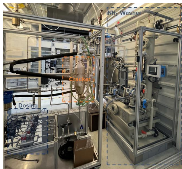
Figure 9: Experimental test setup including the dosing section with MFCs, the catalytic ammonia cracker and an ammonia washer.
