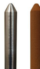
Figure 2. Steel corrosion test as per ASTM D665 for 30:70 Off-spec FAME 3:VLSFO versus clean rod (Left rod).
