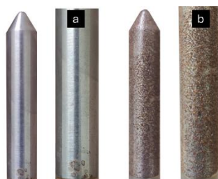
Figure 5. Steel corrosion test showing the effect of aging on corrosion. This test was performed according to ASTM D665 for a. B100 unaged showing no corrosion & b. B100 aged at 43°C for 12 weeks showing significant corrosion.
