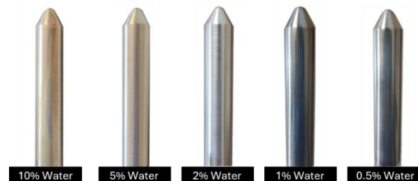
Figure 4. Steel corrosion test showing the effect at different water concentrations for RF2 according to the modified ASTM D665. Rust formation is present at 5% and 10% water concentrations.
