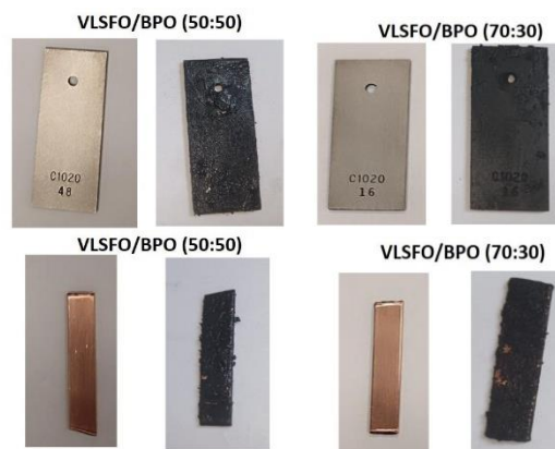
Figure 8 VLSFO / BPO metal specimens, each pair shows the specimen before conditioning on the left and after conditioning on the right.
