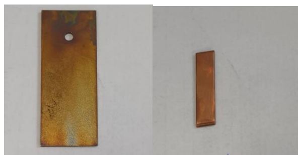
Figure 15 VLSFO/RME B30 metal specimens after conditioning
