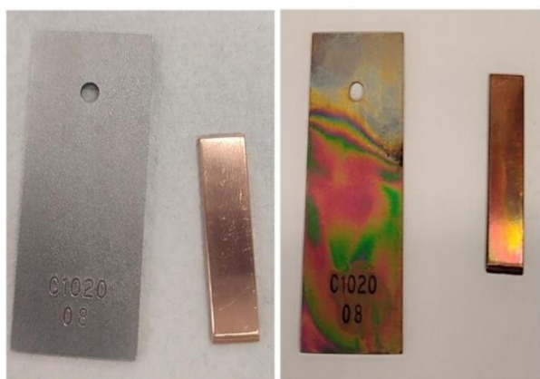
Figure 2 Metal specimens VLSFO, before conditioning shown on the left, after conditioning on the right.
