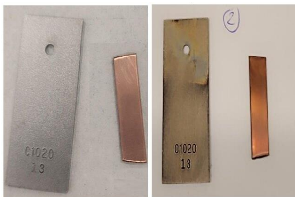
Figure 5 Metal specimens HFO, before conditioning shown on the left, after conditioning on the right.
