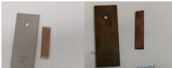
Figure 16 HFO/RME B50 metal specimens before and after corrosion
