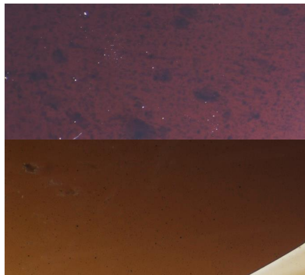
Figure 7 Microscopic evaluation of the B30 VLSFO/BPO blend before conditioning (top) and after conditioning (bottom)
