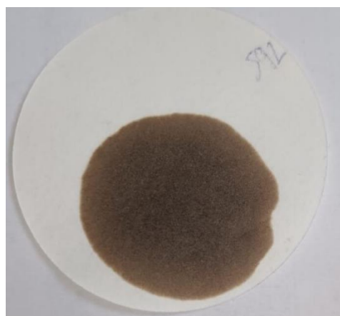
Figure 12 VLSFO/rCNSL B30 blends spot test before and after conditioning
