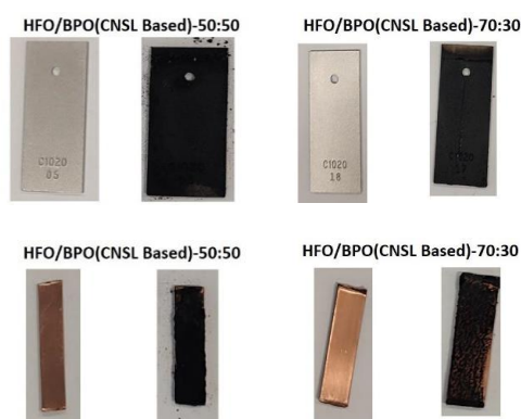
Figure 9 HFO / BPO metal specimens, each pair shows the specimen before conditioning on the left and after conditioning on the right
