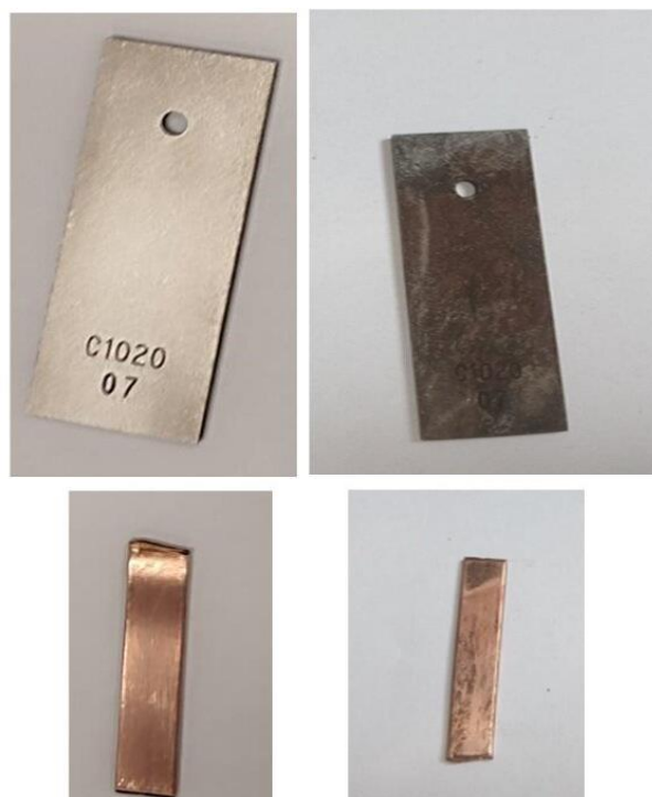
Figure 4 Metal specimens BPO, before conditioning shown on the left, after conditioning on the right.
