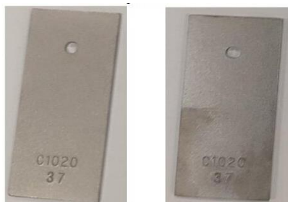
Figure 14 HFO/rCNSL Steel specimen before (left) and after (right) conditioning
