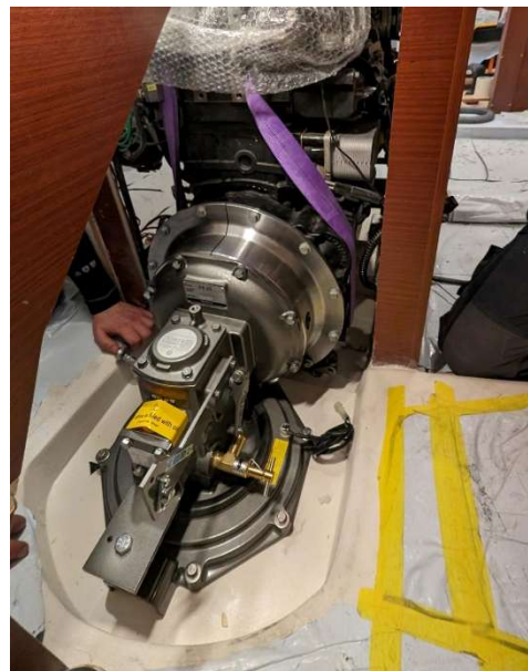
Figure 17. Installed engine and sail drive onboard the yacht
