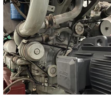
Figure 7 ICE test bench equipped with active PMSM
