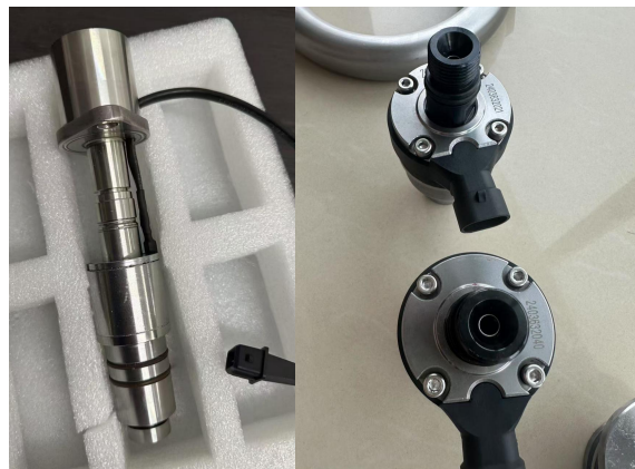
Figure 4. Inlet port methanol injector
