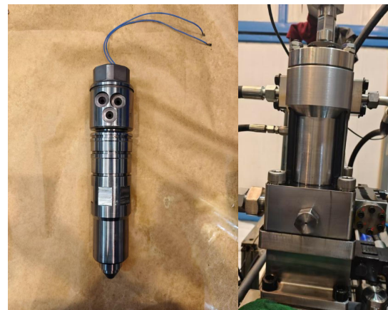
Figure 29. The sample of the methanol-diesel dual-fuel injector and booster pump
