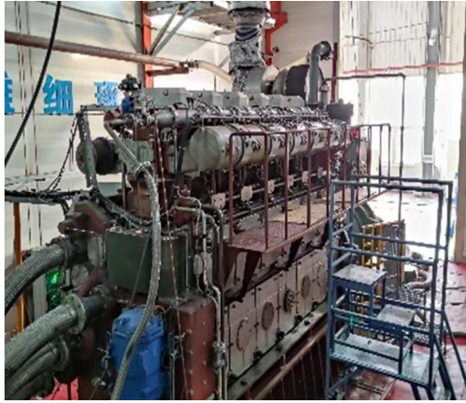
Figure 5. CPGC M320DM low pressure inlet port fuel Injection methanol-diesel dual fuel engine real shot
