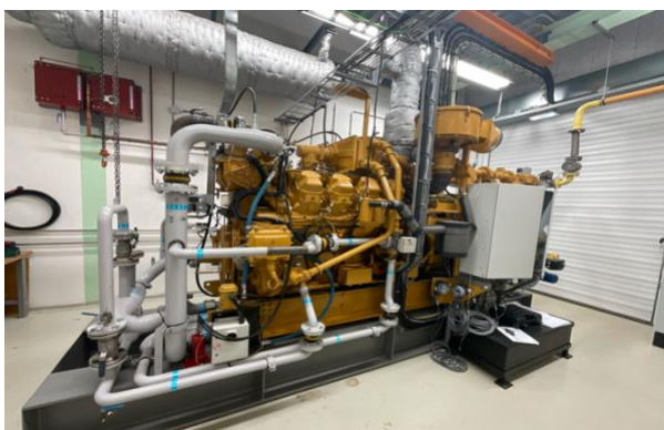
Figure 1 The marine four-stroke NG-SI engine at the NLDA lab, in Den Helder
