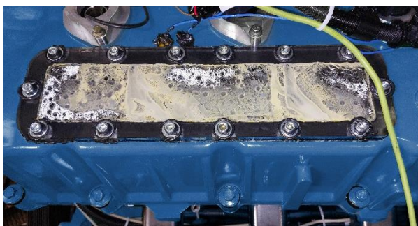
Figure 13: Emulsion formation in valve cover through gauge glass
