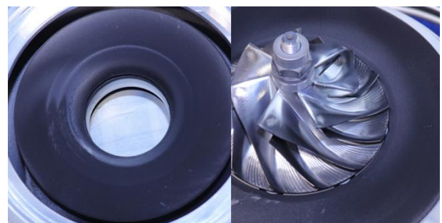
Figure 15: Volute and impeller of compressor after fouling test with closed breather system
