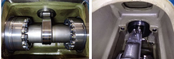
Figure 32 shows the condition of the Camshaft & Crankcase at the end inspection
