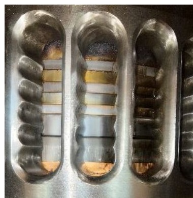
Figure 45 picture shows the good piston condition at 8300 running hours, taken during scavenging port inspection
