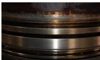
Figure 26 shows the very clean piston ring grooves and ring lands condition at end of test on FAME
