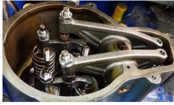
Figure 31 show the condition of the Rocker Arm at end inspection
