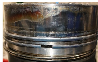
Figure 25 shows the excellent cleanliness of the pistons condition at the end of test on FAME
