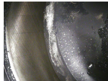
Figure 36 shows the condition of the piston crown top and Cylinder Liner surface at TDC, observed by endoscope
