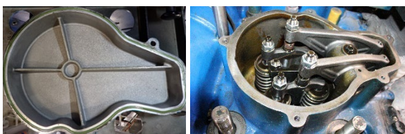
Figure 21 shows the clean condition of the cylinder Head Cover and Rocker Arm at FAME EOT
