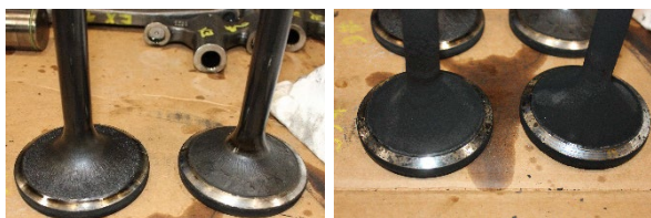
Figure 22 shows the good condition at end of test on FAME operation
