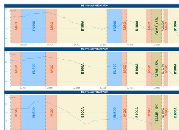
Figure 2 shows the viscosity @40°C trending of all 3 engines when switching between B100 FAME and MGO/EN590
