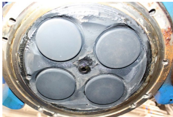
Figure 23 shows minimal deposit formation at end of test on the cylinder Head fire face
