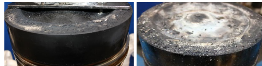
Figure 24 shows the comparison of the piston crown top on Diesel (picture on the left hand side) and FAME operation (picture on the right hand side)
