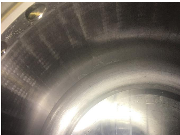
Figure 21: Condition of hydraulic bore in crosshead pin
