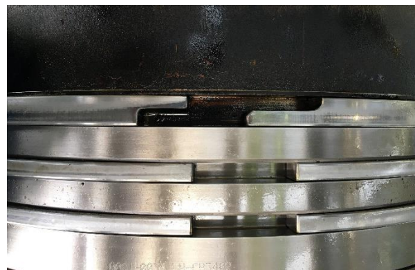
Figure 18: Condition of piston ring pack
