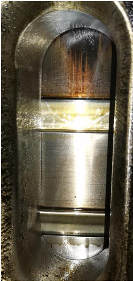
Figure 9: Part of piston head with two piston rings of a WinGD 7X52DF engine after 22'700 operating hours seen through inlet port (by 19.11.2024)
