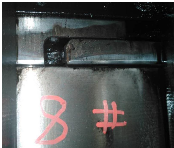
Figure 10: Damaged gas-tight top piston ring lock after workshop operation
