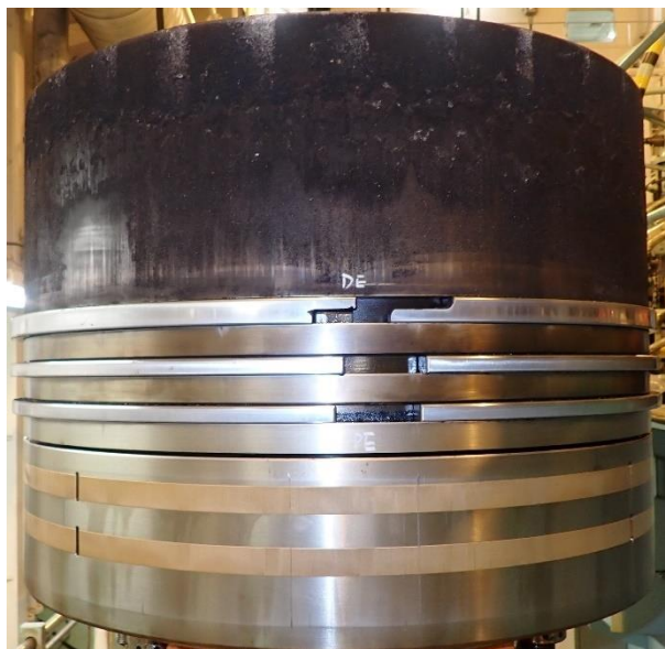
Figure 6: Piston head with three piston rings of a WinGD 9X82 engine after 55'001 operating hours on heavy fuel oil without overhaul (by 01.09.2024).
