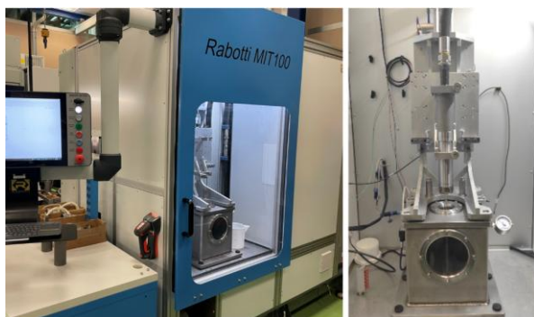
Figure 3: PFI injector test bench ( left ), detailed view of the injection chamber ( right ).
