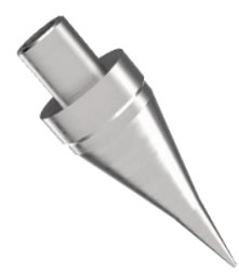
Figure 13. Deflector geometry for big power output
