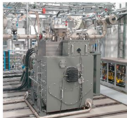
Single-cylinder research engine FM18
