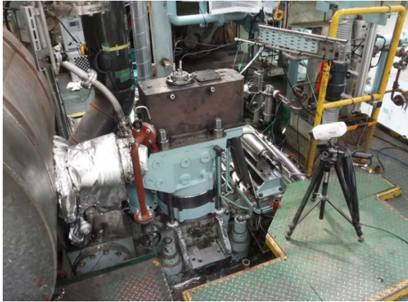
Figure 4 A picture of a single-cylinder test engine
