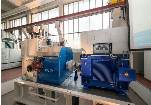
Figure 14. Test engine Caterpillar MaK M34DF-SCE / 4stroke, Source: LKV laboratory of the University of Rostock
