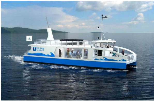
Figure 2. 3D rendering of the 350kW PEMFC ship
