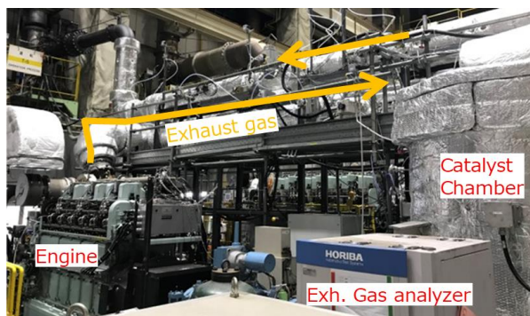
Figure 17. Picture of the actual layout of CH 4 oxidation catalyst.
