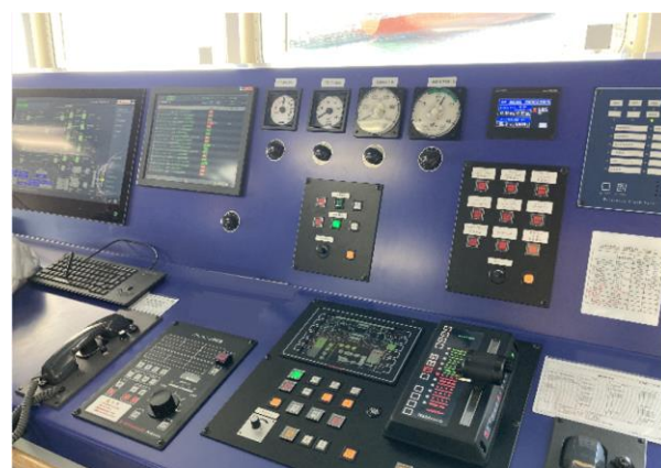
Figure 11. PCS installed on bridge console
