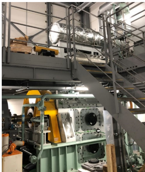
Figure 15. A photo of the single-cylinder test engine
