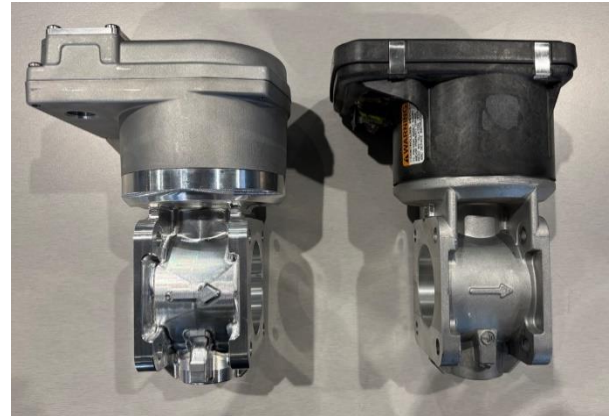
Figure 11. X-Series 68 mm CBV prototype next to an LAT based F-Series CBV.
