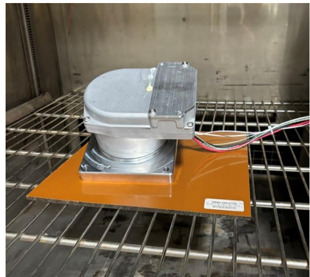
Figure 4. X-Series undergoing thermal testing at Woodward's technology campus.
