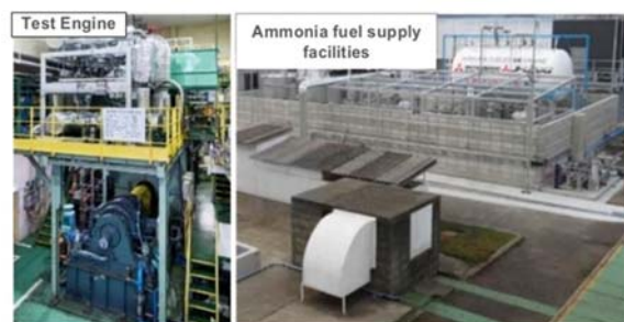
Figure 13. Ammonia-fueled test engine, ammonia fuel supply facilities.
