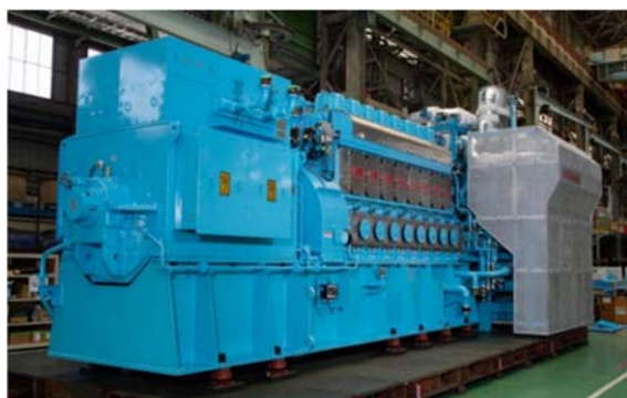
Figure 3. Photograph of KHI's 4-stroke hydrogen-fueled engine 8L30KG-HDF.
