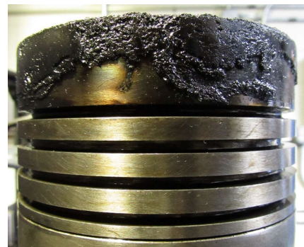
Figure 5. Piston deposits after 18h of ammonia dual-fuel operation on deposit control protocol with average exhaust temperature of 535°C
