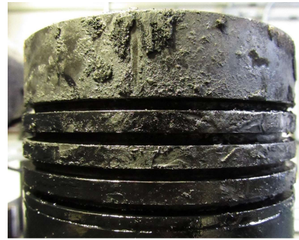
Figure 4. Piston deposits after 65h of ammonia dual-fuel operation at various speed/load conditions. Average exhaust temperatures were approximately 450°C.
