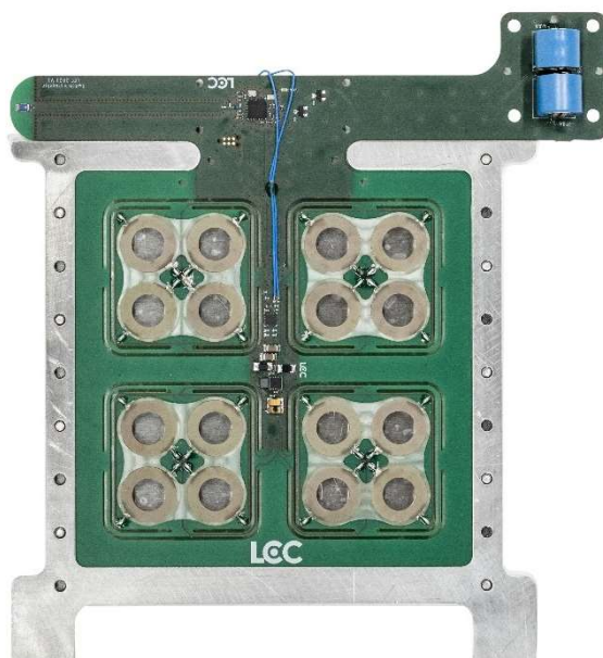
Figure 5: Energy harvesting via piezoelectric elements
