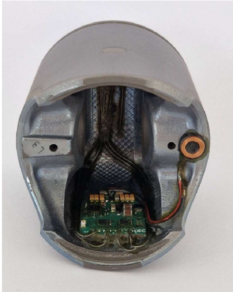
Figure 4: Inductively powered piston temperature telemetry
