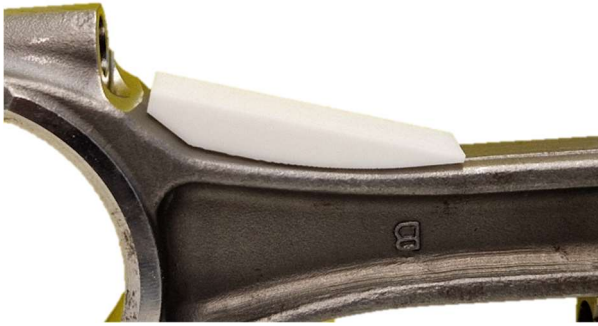
Figure 1: 3D printed dummy for collision check
