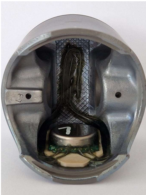
Figure 3: Battery-powered piston temperature telemetry
