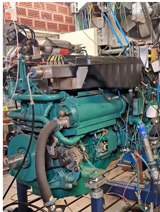
Figure 1. Volvo Penta D16 retrofitted methanol dual-fuel engine installed at VTT.
