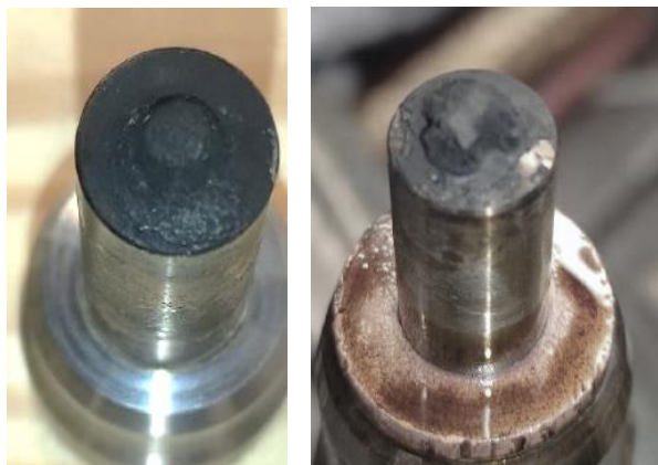
Figure 9: Injector nozzle following engine operation without additive (LHS) and with Additive A (RHS).
