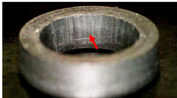
Figure 16. Worn seal element after running
