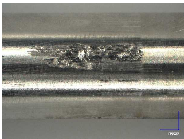
Figure 14. Seizure on sliding parts
