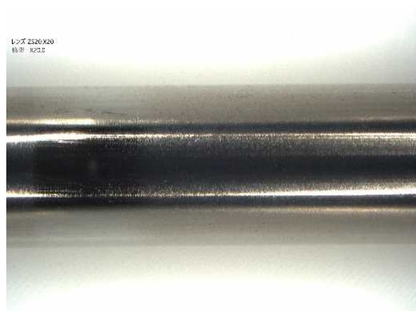
Figure 15. Improved sliding surface with diamond-like carbon (DLC) coating
