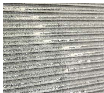
Figure 7. DPF sample was cut to inspect how smoothly ash had accumulated.
