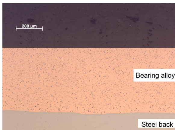
Figure 16 Cross section of Miba 2C (InnoAlloy lead free bronze material)
