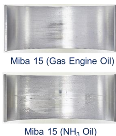
Figure 12 Comparison of a Miba 15 (AlSn-Alloy) test rig bearing running on a fresh gas engine oil and an ammonia aged oil
