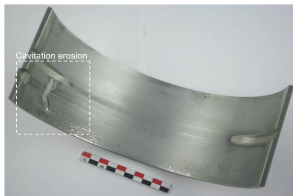
Figure 14 Bearing with severe cavitation erosion
