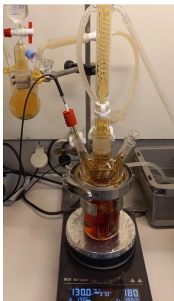
Figure 5 Oil aging tests in laboratory scale
