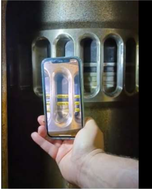
Figure 12. Highlighted yellow boxes indicate successful component image detection – the next step in the process is condition assessment analysis in real time.
