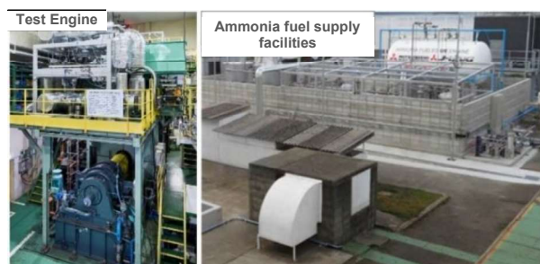
Figure 5. Ammonia-fueled test engine, Ammonia fuel supply facilities
