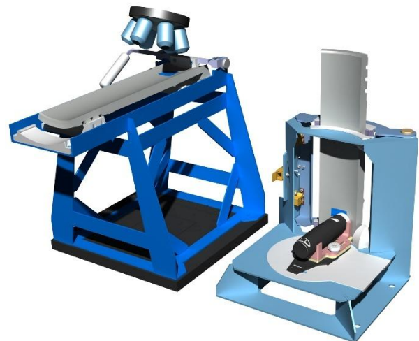
Figure 6: Cylinder liner segment support device for sophisticated stationary reference microscope measurements (left) and liner segment holder for simple handheld microscope measurements (right).
