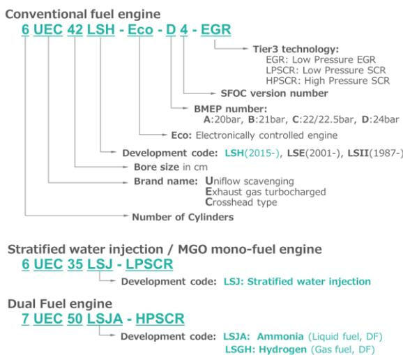
Figure 2. Naming convention of UE engine
