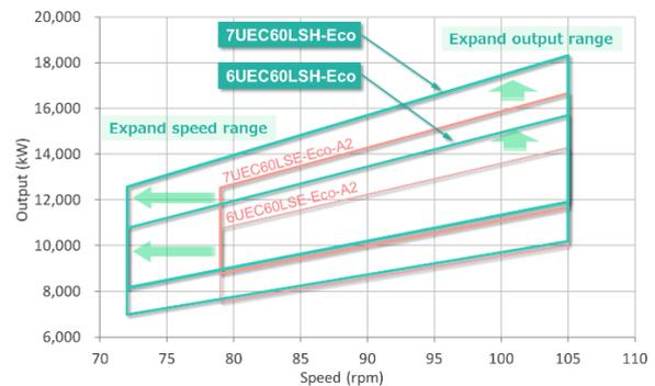
Figure 11. Main specifications and rating map of UEC60LSH-Eco type engine
