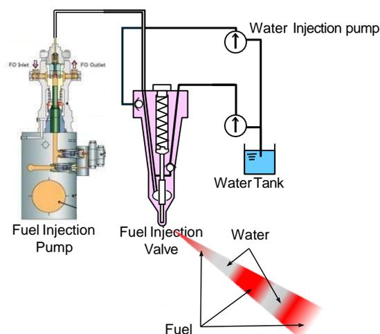
Figure 17. Stratified water injection system
