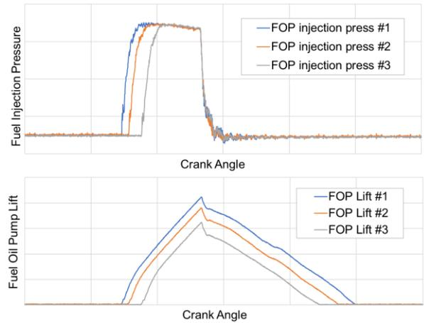
Figure 14. Fuel injection pressure and pump lift of SFOC version 4
