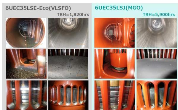
Figure 19. Inspection results on UEC35LSJ (right)
