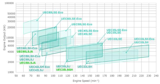
Figure 3. UE engine output x speed range
