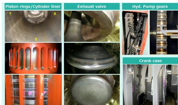
Figure 16. Inspection results on UEC42LSH
