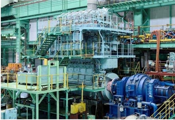
Figure 12. 6UEC42LSH-Eco-D4 type engine
