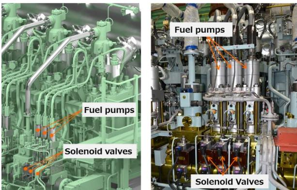
Figure 13. Fuel injection system of SFOC ver. 4
