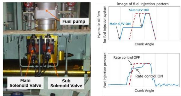
Figure 15. Fuel injection system and injection pressure of conventional engine
