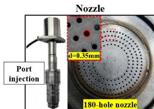
Figure 3. Methanol injector for experiment
