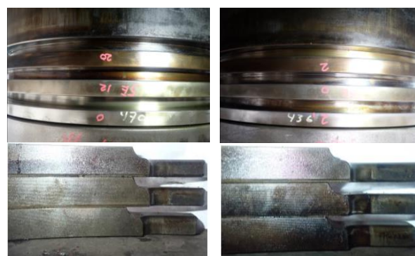
Figure 16. Photographic comparison between piston ring lands and grooves (exhaust side) as well as ring backsides (left: 100BN test oil with Group II EHC 340 MAX™ thickener; right: 100BN reference oil with Group I BS thickener).
