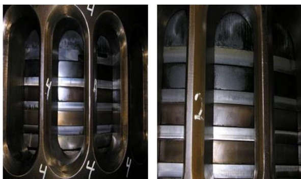
Figure 22. Piston ring pack area cleanliness (left: C9071, right: Reference oil), total piston ring land demerit and drip oil Fe trending of low-viscosity C9071 vs. 70BN fleet commercial reference oil. The average level of sulfur in the fuel oil over this test period is 3.3wt%.
