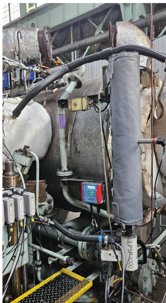
Figure 2. Picture of the mini receiver that was used to sample exhaust gas from the cylinder running on hydrogen. The sample was extracted right after the exhaust valve as shown in the top left of the picture.
