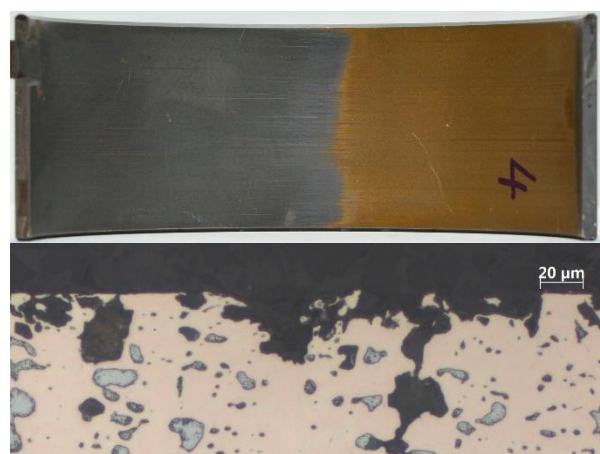
Figure 6. Delamination of the Polymer layer due to lead corrosion at the main loaded area of a conrod upper bearing from a high-speed methanol engine
