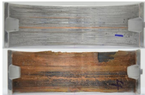
Figure 5. Numerous particles scorings (upper) and seizure (lower) of main bearing lower shells in a high-speed diesel engine
