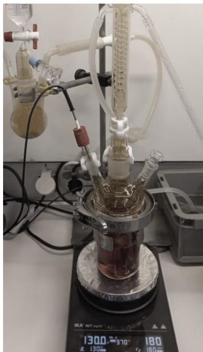
Figure 37. Set up of the artificial oil aging test
