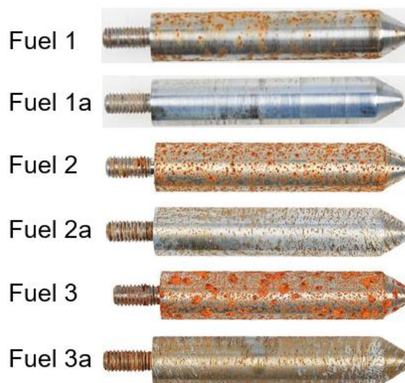
Figure 3. Images of the steel test rods comparing base fuels 1-3 to the additised versions at end of each test.
